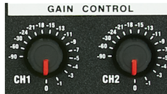
Figure 2.4: Analog Level Controls
