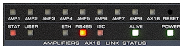
Figure 3.60: SXL II - LED Indicators Front Side
