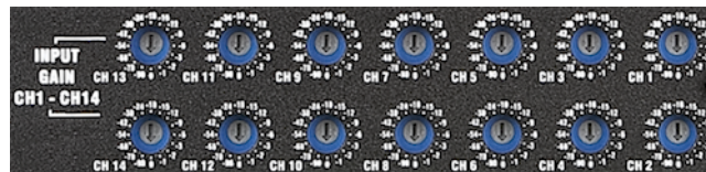
Figure 3.50: AX16 - Digital Level Controls
