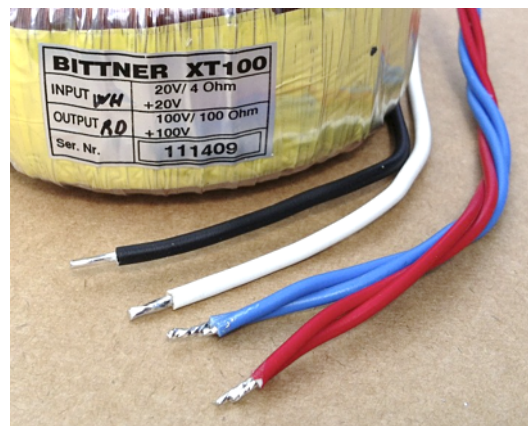
Figure 3.35: XT Transformer - Connection Wires and Sticker
